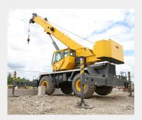
Cummins has presented the advantages of plugin hybrids for applications such as mobile cranes, which use diesel for transport and plug-in power for crane operation [6]. This technology enables silent operation with reduced tailpipe emissions on urban construction sites and fuel consumption is reduced by up to 50% on the overall duty cycle.
